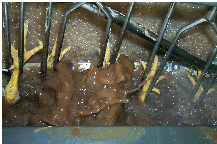
The use of SAS® process water acidifier in the scald is meant to counterbalance the pH increase that occurs due to the presence of fecal material.
